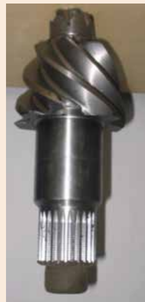
Figure 3: Heavy truck pinion carburized and intensive quenched in AFC-Holcroft UBQ batch carburizing furnace
