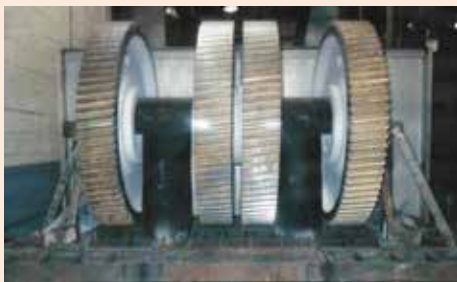
Figure 2: Four 32-in. diameter spur gears carburized and intensive quenched in AFC-Holcroft UBQ batch carburizing furnace.
